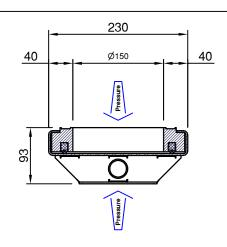
Operation point 1/2 Moon Open / close: ±31 Turns Torque open / close: ±25Nm
